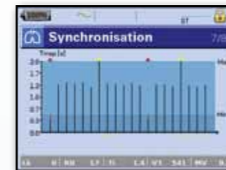
The Synchronisation screen displays spontaneous versus machine-triggered/cycled breaths
